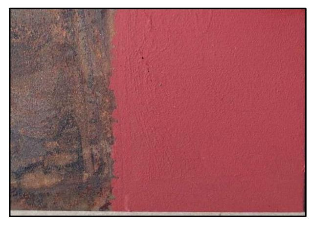
Below an actual sample of rusted steel plate, with a single coat of **Hydro Paint over Rust** applied.
